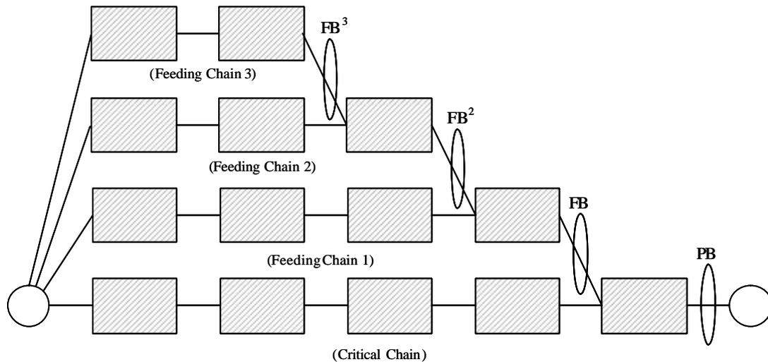
Figure 3 – Feeding buffers at different levels
