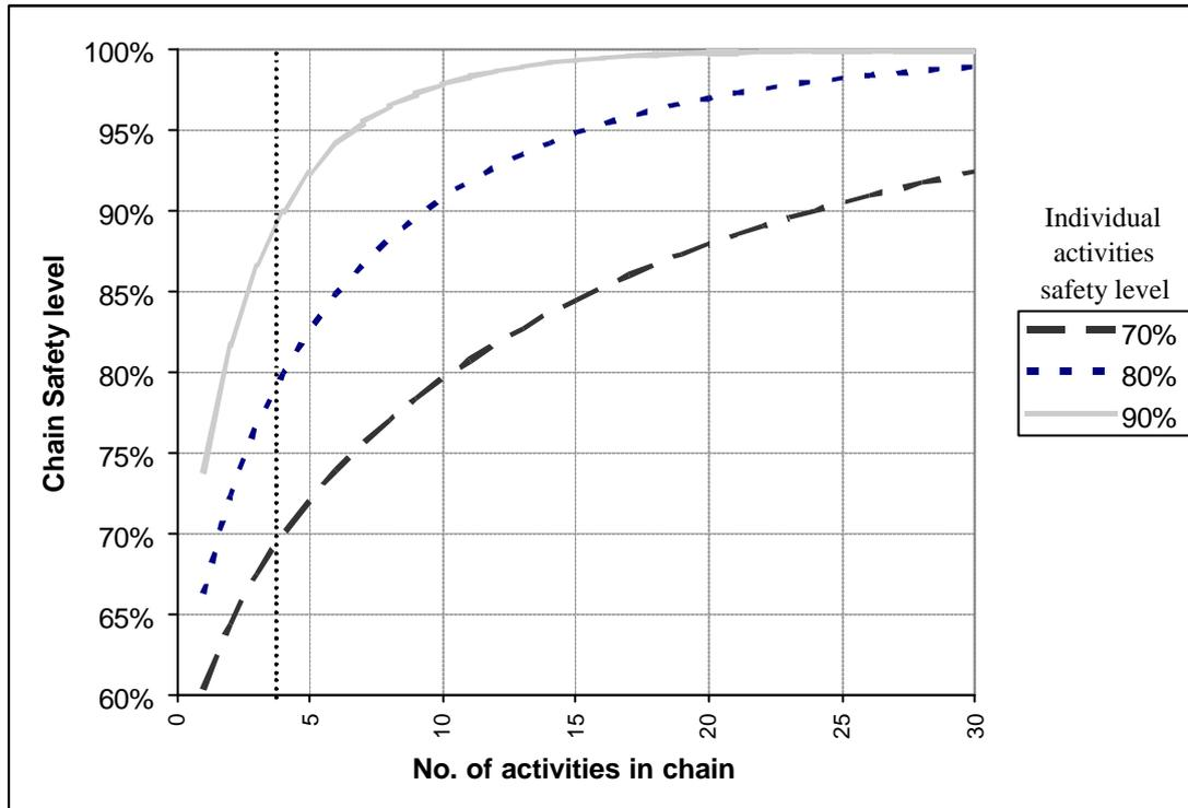
Figure 4 – Chain safety level using Goldratt’s rule of thumb
